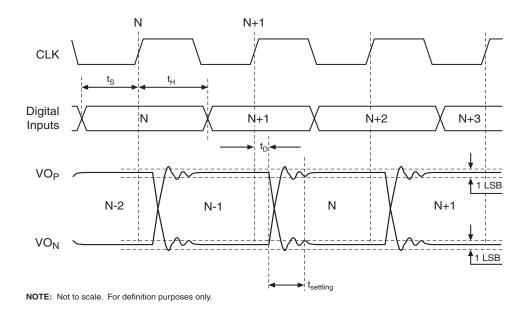
Figure 1: Timing Diagram
